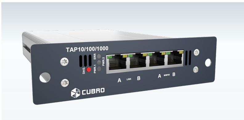
The Cubro 10/100/1000 Copper TAP allows the uninterrupted passage of full duplex data over standard Category 5/6 copper network cable. Featuring auto negotiating between 10Mbps, 100Mbps and 1000Mbps, this TAP duplicates the network signals, including any existing physical errors to the transmit-only monitoring ports.
