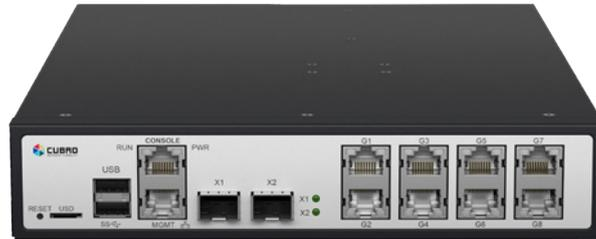
The Cubro Omnia10 is a universal platform that is small in size yet powerful. It can be used for several monitoring applications for the enterprises, lab testing markets, and tactical markets. The main components of this platform are 4 copper links (8 ports) and 2 x 10 Gbit SPF+ ports, a lot of CPU power and memory, USB 3.0 and M2 disc interface internally\*. The copper ports are links safe (TAPs) which enable the device to be used inline.
