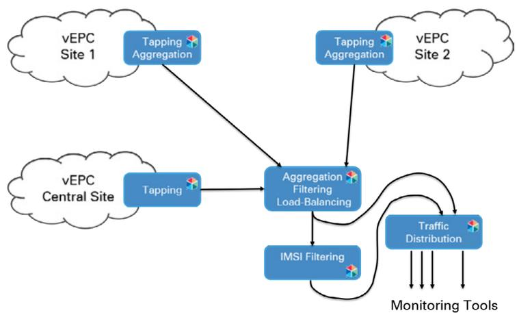
Cubro MTP TAP tapped the traffic and sent it to the Packetmaster EX20400 for aggregation. EX20400 aggregates all incoming vEPC traffic of site 1 and 2 (user and signalling) and load-balances it by means of five tuple hashing. The next steps included aggregation, filtering and load balancing.
