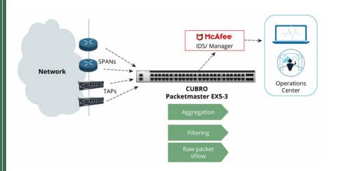
Besides raw packet forwarding, the EX5-3 produces also sflow information and sends it the IDS for further checks.
