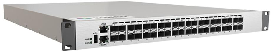
The Sessionmaster EXA40 Series is the next evolution step in the row of the successful Cubro network packet broker product line. The Sessionmaster handles packets up to layer 7 and load balances based on specific applications. The possibility to do keyword and regular expression searches, completes the big picture of the EXA and allows it to fit into almost every situation in monitoring systems.
