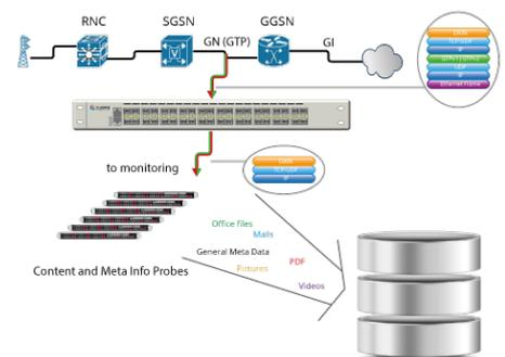
It is a two-stage concept; typically the GN ports carry much traffic up to multiple 10 Gbps. Therefore it must split the traffic into smaller portions. The first stage is to load balance the traffic session aware to 20 Gbps portions. In the second step, the Sessionmaster EXA24160 correlates the GTP traffic (4 tunnels) and search for the IMSI in the signalling tunnel. The information in the signalling tunnel provides the transport information to find the customer traffic in the data tunnels.
