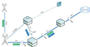
These applications show the capability of the Sessionmaster EXA24160 to filter inside the GTP tunnel without removing the GTP header. The application is filtering the HTTP traffic inside the tunnel and load balance the traffic. As an additional feature, the GTP header could also be removed from the filtered traffic.
