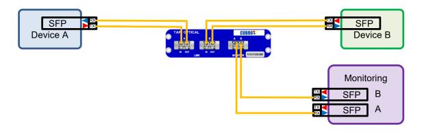
Note: There is no need to take LC duplex connectors apart, cables can stay in the original state.
