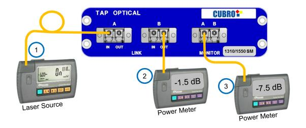
Typical attenuation values including connector loss:
