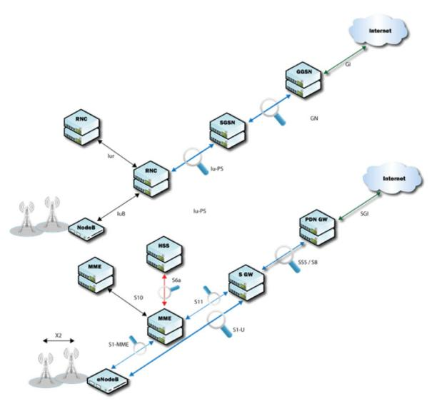
The network in this image is monitored using monitoring probes. The probe is connected via a TAP network and aggregation devices (network packet brokers) to the different interfaces on the network. These interfaces are logically and physically distinct which allows us to get a full view of what's going on in the network. Probes analyze all of these different interfaces.
