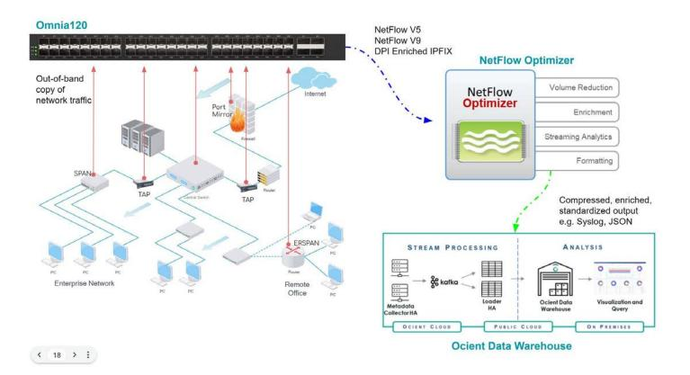
As in the example above combination of Cubro TAPs and mirror ports (such as SPAN and ERSPAN feeds) provide a copy of all network traffic to an Omnia120. The Omnia120 generates DPI enriched IPFIX records from all traffic sessions. These records are sent to a local instance of NetFlow Optimizer for processing, aggregation, and further data enrichment. The output is standardized and sent to a remote centralized installation of Ocient Data Warehouse for retention and analysis.
