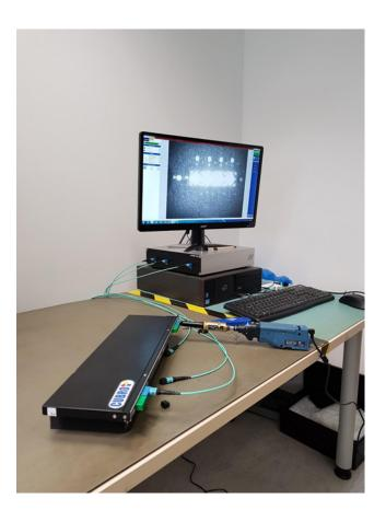
Cubro has developed a proprietary measurement device (1), that can measure up to 4 fiber pairs simultaneously, using all bandwidth speeds and all wavelength frequencies. This measurement method is not only very fast but produces repeatable results on each link; this is not often the case with standard optical power meters. The reason for this is that optical power meters are normally designed to measure longer optical fibers and not those of a very short distance.
