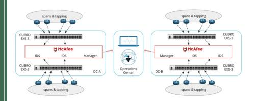
Relevant network traffic from all span ports and tapping points is aggregated and provided to McAfee Security solution. A central operation center is thus able to analyze this traffic and to keep the network safe.
