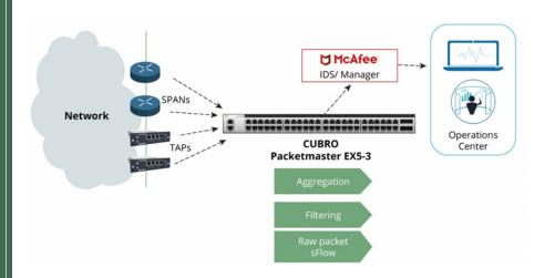
Besides raw packet forwarding, the EX5-3 produces also sflow information and sends it the IDS for further checks.
