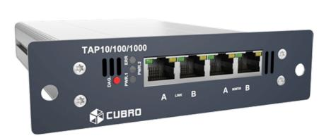
The Cubro Ethernet 10/100/1000Mb Copper TAP allows the uninterrupted passage of full duplex data over standard Category 5/6 copper network cable. Featuring auto negotiating between 10Mbps, 100Mbps and 1000Mbps, this TAP duplicates the network signals, including any existing physical errors to the transmit-only monitoring ports.
