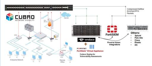
EndaceProbe™ Analytics Platforms capture, index and store network traffic with 100% accuracy, regardless of network speeds, loads or traffic types. This recorded Network History provides the definitive evidence that helps the SecOps and NetOps teams to quickly and accurately investigate and respond to security threats and performance issues.
