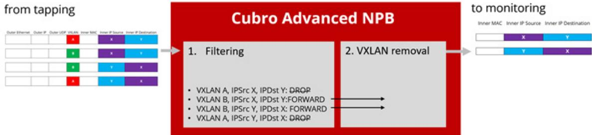
VXLAN VNI and inner IP filtering:
