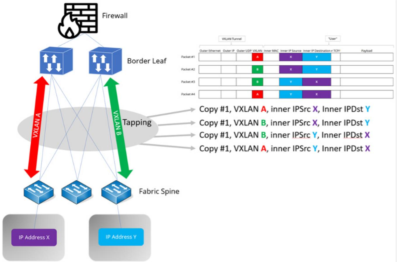
Traffic between IP X and IP Y passes the tapping two times and thus the same packets are visible twice at the tapping output. From user perspective every packet is received twice. The EXA64100 offers an easy and straight-forward way to eliminate the duplicates by allowing filtering VXLAN VNI and inner IP simultaneously.
