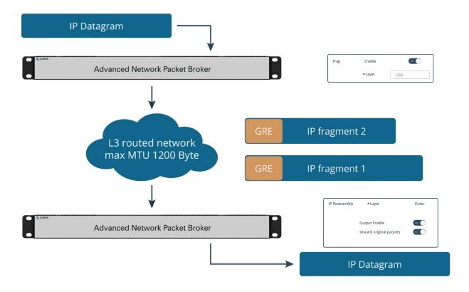
IP fragmentation is the process of breaking down a large IP datagram (packet) into smaller pieces, called fragments, to fit across network links with a smaller Maximum Transmission Unit (MTU) size. The EXA48800 supports fragmentation to any selectable MTU size between 512 Byte and 2048 Byte. In addition, fragmented packets can be encapsulated into a GRE tunnel to be transmitted over a routed Layer 3 network.
