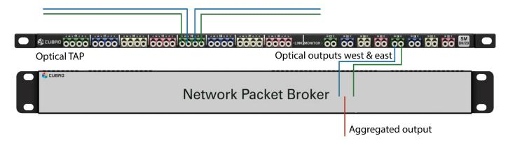
By utilizing the various filtering capabilities of the EXA48800, the user is able to further reduce traffic volume that needs to be processed, thus enabling quicker and more accurate analysis and troubleshooting. Moreover, incoming traffic can be VLAN tagged per physical port to allow easy identification at which physical port a packet original arrived.
