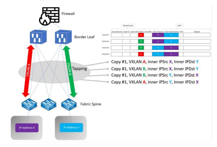
Traffic between IP X and IP Y passes the tapping two times and thus the same packets are visible twice at the tapping output. From user perspective every packet is received twice. The EXA32400 offers an easy and straight-forward way to eliminate the duplicates by allowing
