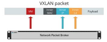
Every port of the EXA32400 supports an independent MAC and IP setup. Thus, the EXA32400 can be used as an active tunnel endpoint. Beside tunnel termination it also allows filtering inside tunnels.
