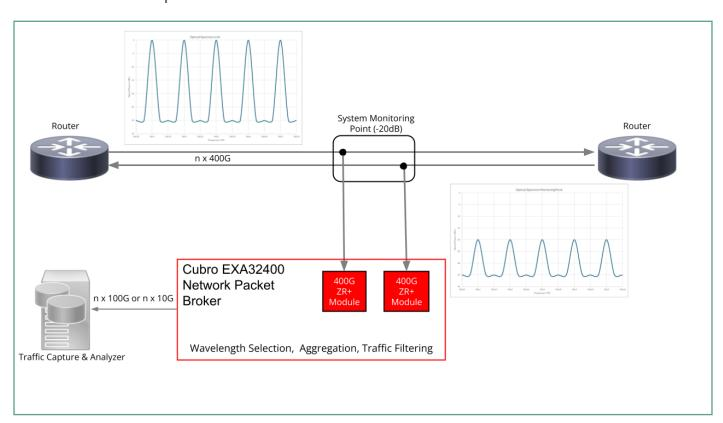
The Cubro EXA32400 Network Packet Broker connects directly to the DWDM system via protected monitoring points, providing a non-intrusive way to access live optical signals. Using QSFP-DD ZR+ tunable modules, engineers can precisely select the wavelength of the 400G signal that needs to be analyzed, enabling targeted traffic capture without disrupting production traffic.
