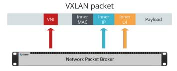
Every port of the EXA32100A supports an independent MAC and IP setup. Thus, the EXA32100A can be used as an active tunnel end-point. Beside tunnel termination it also allows filtering inside tunnels.
