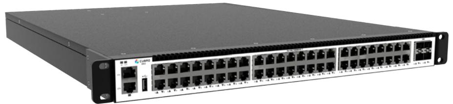
The Packetmaster EX5-3 is Cubro's first Hybrid Network Packet Broker. It combines a packet broker with traditional features of a network switch. This unique setup makes the solution more flexible compared to conventional solutions where each component is a separated hardware. The unit can be used inline and filter out specific traffic and send it to a probe.
