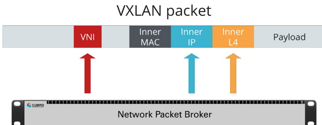
Every port of the EX48800 supports an independent MAC and IP setup. Thus, the EX48800 can be used as an active tunnel end-point. Besides tunnel termination, it also allows filtering inside tunnels. This superior functionality makes the EX48800 perfectly suited for any modern overlay network.
