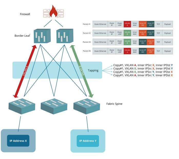
Traffic between IP X and IP Y passes through the tap twice, causing the same packets to appear twice at the tap output. From the user's perspective, each packet is received twice.
