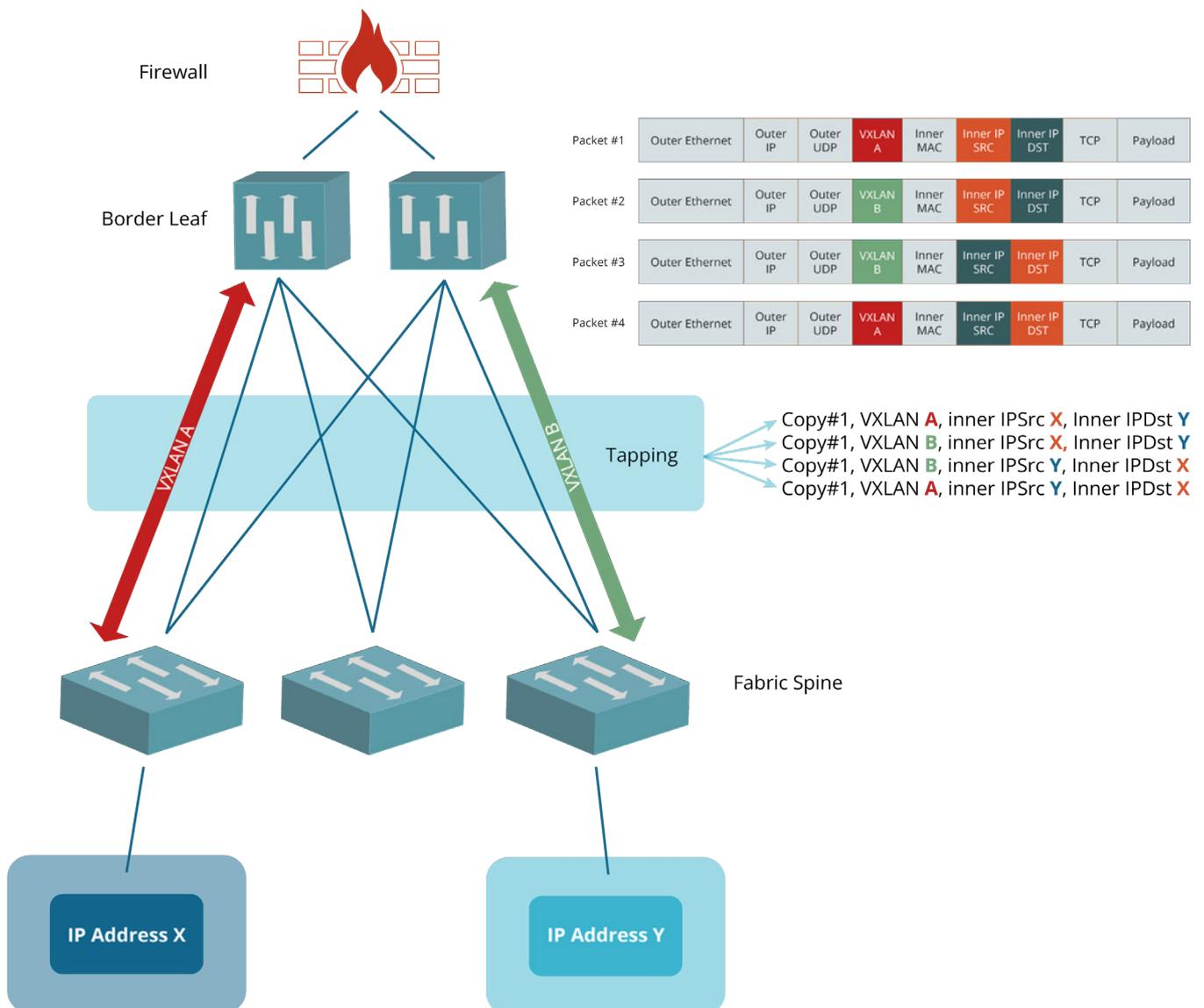
Traffic between IP X and IP Y passes through the tap twice, causing the same packets to appear twice at the tap output. From the user's perspective, each packet is received twice.
