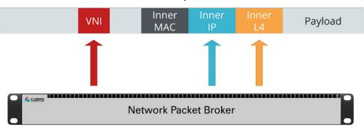
Every port of the EX48800 supports an independent MAC and IP setup. Thus, the EX48800 can be used as an active tunnel end-point. Besides tunnel termination, it also allows filtering inside tunnels. This superior functionality makes the EX48800 perfectly suited for any modern overlay network.
