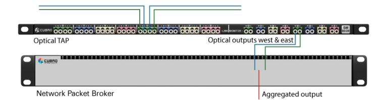
By utilizing the various filtering capabilities of the EX48200, the user is able to further reduce traffic volume that needs to be processed, thus enabling quicker and more accurate analysis and troubleshooting.
