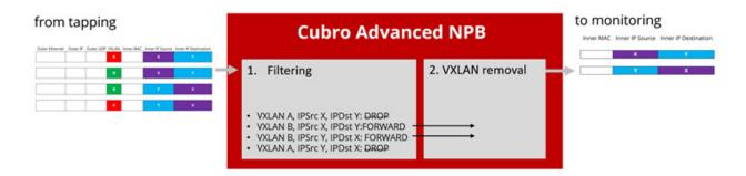
From user perspective the setup of the filtering and VXLAN removal should be as simple as possible. Following screenshots from Cubro Advanced NPBs show the easy and fast setup for filtering and VXLAN removal.
