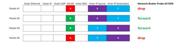
The advanced Packet Broker enables all the required filtering (VXLAN & inner IP) and also removes the outer VXLAN tunnel before sending the packets to the monitoring system. This way output traffic to the monitoring system does not include any duplicates and has pure "user-data" without VXLAN encapsulation.
