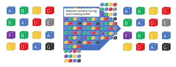
Automatically adjusting time window will have lower window size when the number of packets grows (bandwidth grows and/or packet size decreases) to ensure best possible deduplication performance. Of course, it will not detect duplicates if the network delivers duplicate packets outside the used time window.
