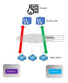
Traffic between IP X and IP Y passes the tapping two times and thus the same packets are visible twice at the tapping output. In detail, traffic on tapping output looks like this:
