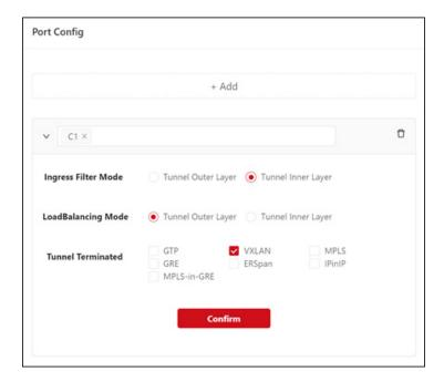
Filter based deduplication is very efficient and it doesn't require additional resources if the NPB supports it. The downside is that the network topology needs to be known.
