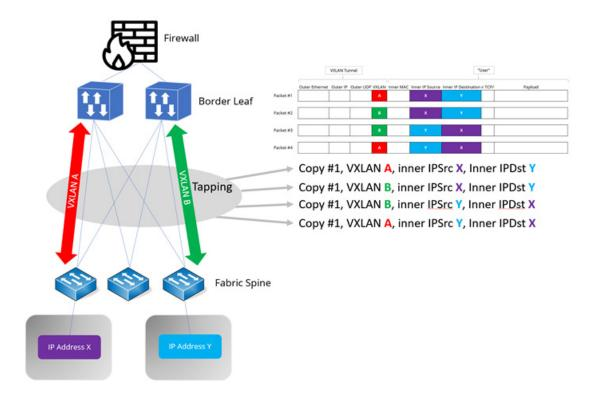
An easy and straight-forward way to eliminate the duplicates is to use a combination of **VXLAN VNI and inner IP filtering**.
