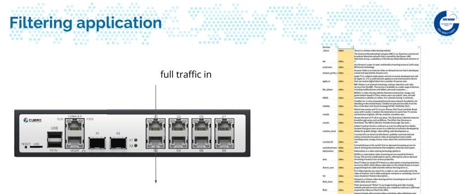
Traffic out without video stream traffic to reduce load on monitoring or capture device
