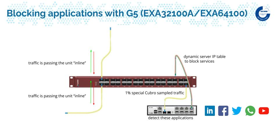
The detector can be any CPU based unit, also a server.
