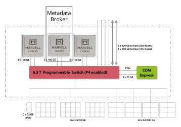
In this case one CPU is used to run the Metadata Broker to feed results direct to any other tool
