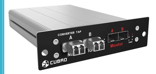
The Cubro Converter TAP is a flexible solution to convert interfaces for tapping purpose. The Converter TAP is available in 2 different versions, fixed optical link ports (SM or MM) with SFP monitor ports or SFP Link ports with fixed monitor ports (SM or MM). The second one is called R version.
