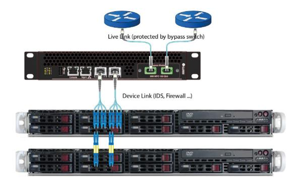
**Bypass Application – Load Balancing**
