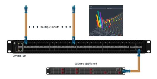
The Cubro solution helps to offload the capture appliance and at the same time delivers a DPI metadata view of the full traffic in all details, with a bandwidth resolution in 1 sec. This data can also be used for further analytics.
