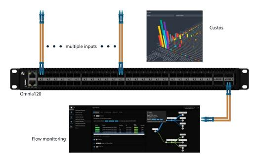
The Cubro solution helps to offload the NetFlow appliance and at the same time delivers a DPI metadata view of the full traffic in all details, with a bandwidth resolution in 1 sec. This data can also be used to enrich the flow data. The main advantage is that Custos handles the traffic, which is poison for Flow solutions. Cloud services with millions of flows.
