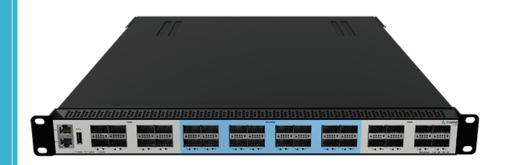
The Aggregator C32 is a high-performance network packet broker that aggregates, filters, duplicates, load balances network traffic to security, monitoring and management tools based on 4000 possible rules. The Aggregator C32 supports OSI Layer 2, Layer 3 and Layer 4 header modifications including stripping, adding, and modifying VLAN tags, MAC addresses, IP addresses and Port numbers.
