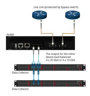
The output for the inline device load balanced is 4 x 25 Gbit or 4 x 10 Gbit.
