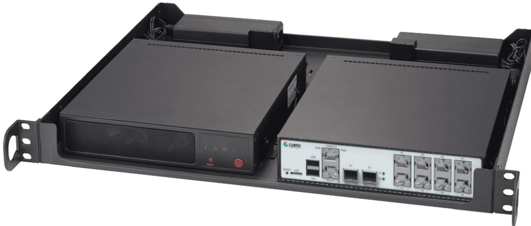
The EXA8 comes in combination with a flow collector. The flow collector is a standard server with a collector software. There are several collector software applications, commercial and open source, available on the market.
